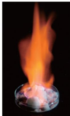
Methane hydrate (artificial) burning
